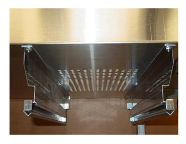
Position the CORN DRAWER SUPPORTS so that the CLEAN OUT DRAWERS may be slid between them, right beneath the table as shown. Screw the four CORN DRAWER SUPPORTS onto the table, each SUPPORT requires two 1/4-20 x 1/2 CARRIAGE BOLTS and two 1/4-20 SERRATED HEX FLANGE NUTS. Note: There are no washers needed. Insert the BOLTS from the top of the table, and tighten the HEX FLANGE NUTS on the SUPPORT sides.
