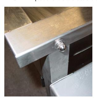
2. Using two 1/2-13 x 2 1/4 BOLTS, two 1/2-13 HEX NUTS, and two 1/2 SPLIT WASHERS, attach the top bolts to hold the SHELF in position, using the topmost holes beneath the SHELF. Insert the BOLTS from the inside of the TRAY, and secure the BOLTS with the SPLIT WASHERS and HEX NUTS beneath the SHELF.
